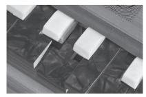
and lift the keyboard. Turn the keyboard over to see the underside of the keys. Each key will have a bent wire that acts as a spring arm. Find the offending key and reset the spring arm into place. In the photo to the left the center key has a slipped spring arm.
